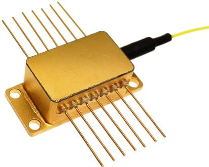
Single mode FBG-stabilized laser diode module designed for optical measurement and communication. The laser is packaged in Butterfly package with monitor photodiode and thermo-electric cooler (TEC). Module is pigtailed with 0.5-0.9 m of single mode or polarization maintaining (optional) fiber and connectorized by FC/APC connector.
