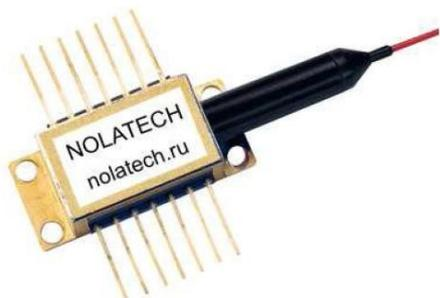
TLD-1310-14BF Fiber Bragg Grating laser is a stable narrow band light source with a wavelength tuning possibility in 1-2 nm range. The laser is packaged in 14-pin standard butterfly package with monitor photodiode and thermo-electric cooler (TEC).
