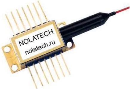
SLD-910-14BF Superluminescent Diode is a light source for fiber transmission systems, fiberoptic gyros, fiberoptic sensors, optical coherence tomography, optical measurements. The diode is packaged in 14-pin standard butterfly package with monitor photodiode and thermo-electric cooler (TEC). Module is pigtailed with 0,7-1,0 m of single mode polarization maintaining fiber and connectorized by FC/APC connector.
