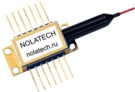
SLD-680-14BF Superluminescent Diode is a light source for fiber transmission systems, fiberoptic gyros, fiberoptic sensors, optical coherence tomography, optical measurements. The diode is packaged in 14-pin standard butterfly package with monitor photodiode and thermo-electric cooler (TEC). Module is pigtailed with 0,7-1,0 m of single mode polarization maintaining fiber and connectorized by FC/APC connector.
