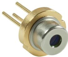
SLD-1550-9MM-50 double-pass superluminescent diode is a light source for fiber transmission systems, fiberoptic gyros, fiberoptic sensors, optical coherence tomography, optical measurements. The diode is packaged in standard 9mm TO can.
