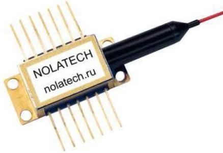
FPL-950-14BF is single mode laser diode module designed for optical measurement and communication. The laser is packaged in 14-pin standard butterfly package with monitor photodiode and thermo-electric cooler (TEC). Module is pigtailed with 0,7-1,0 m of single mode polarization maintaining fiber and connectorized by FC/PC connector.
