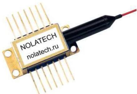
FPL-740-14BF is single mode laser diode module designed for optical measurement and communication. The laser is packaged in 14-pin standard butterfly package with monitor photodiode and thermo-electric cooler (TEC). Module is pigtailed with 0,7-1,0 m of single mode polarization maintaining fiber and connectorized by FC/PC connector.
