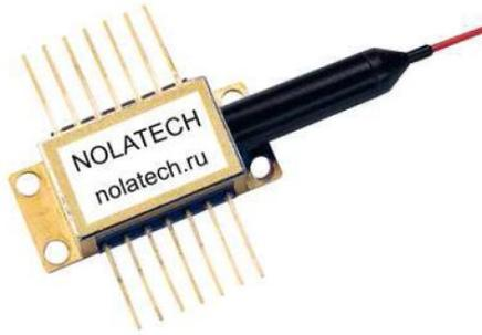
FPL-1650-14BF-200 is single mode laser diode module designed for optical measurement and communication. The laser is packaged in 14-pin standard butterfly package with monitor photodiode and thermo-electric cooler (TEC). Module is pigtailed with 0,7-1,0 m of single mode polarization maintaining fiber and connectorized by FC/PC connector.
