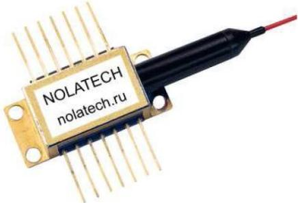
BLD-1550-14BF Fiber Bragg Grating laser is single frequency laser diode module designed for optical measurement and communication. The laser is packaged in 14-pin standard butterfly package with monitor photodiode and thermo-electric cooler (TEC).
