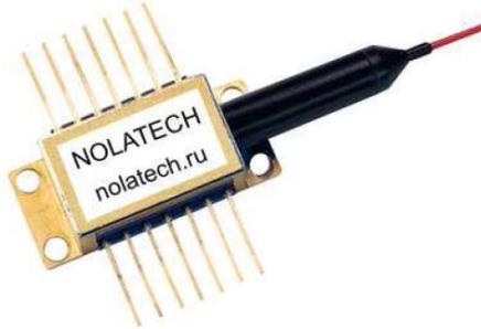
FPL-FBG-1300-14BF-10 is FBG-stabilized laser diode module designed for optical measurement and communication. The laser is packaged in 14-pin standard butterfly package with monitor photodiode and thermo-electric cooler (TEC). Module is pigtailed with 0,7-1,0 m of single mode polarization maintaining fiber and connectorized by FC/APC connector.
